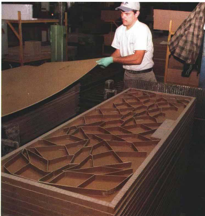
Hollow-core doors assemble in a snap. After gluing the stile, rails and lock block to one hardboard skin, workers unfold corrugated cardboard onto the center of the door and lay the second skin down; the entire process takes less than ten seconds.
